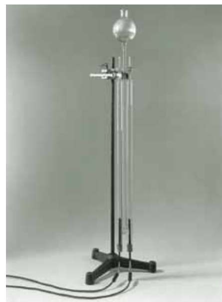
Water decomposition apparatus named after A.W. Hofmann (1818–1892), still in use today (photo: Deutsches Museum, Munich, Germany).
