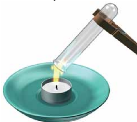
A combustible gas
