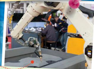
The area defined by all of the positions in space that the end of the robotic arm can reach is known as the workspace. If the object that the robotic arm needs to pick up is not in the workspace, the robot cannot pick it up! The workspace depends on the degrees of freedom, limitations of the joints, lengths of the linkages, and the angles at which the object must be picked up.
