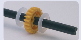
Plastic washers can be used to separate gears.
