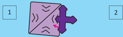
Connecting the tiles with the connectors (the plus-sign shaped pieces)
