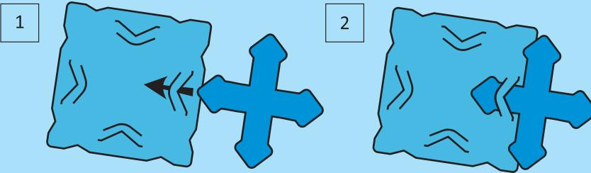
Connecting the tiles with the connectors (the plus-sign shaped pieces)
