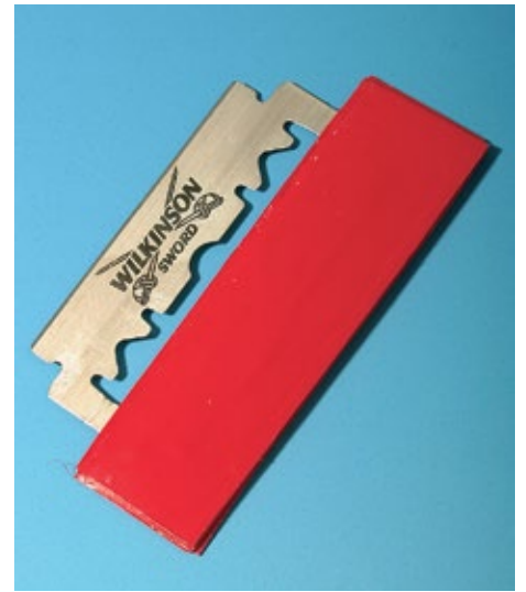
The insulating tape grip greatly reduces the danger of injury.
