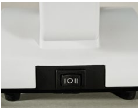
The light switch for incident light (II) and transmitted light (I)
