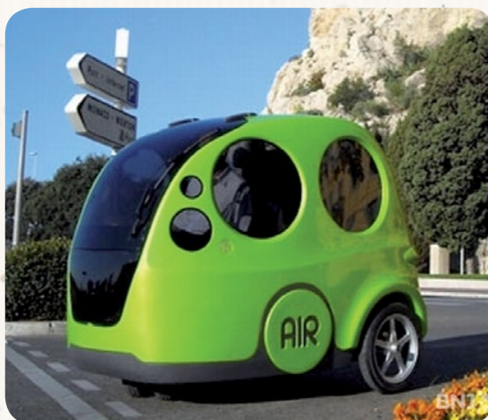
The car of the future? This futuristic car is called AirPod, and it can go about 200 km on a tankful of compressed air.
