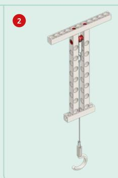
Here, use a piece of string about 20 cm in length. Tie the lower end to the hook. At the top end, tie a loop and hang it on the spring.
