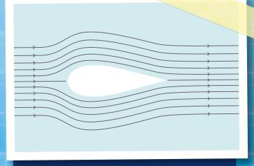
The path of streamlines is especially important for airplane wings, helicopter rotor blades, and wind turbines, since they determine how stable the plane will be in the air or how efficient the wind turbine will be.
