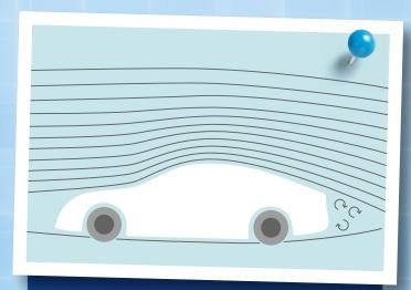
A car's fuel consumption at high speeds is strongly influenced by how streamlined it is. That's why a car prototype is often tested in a wind tunnel as a new model is being developed, to make sure that it has a streamlined shape and so that adjustments can be made if it doesn't.
