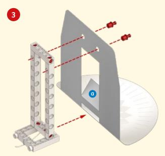
Part (a) will have to be folded down, with the exact angle depending on the location of the sundial, to increase the amount of light.
