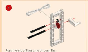
gear wheel before inserting the axle,
