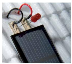
2. Position the Power House so that sunshine hits its solar cell. The LED lights up and the motor runs.
