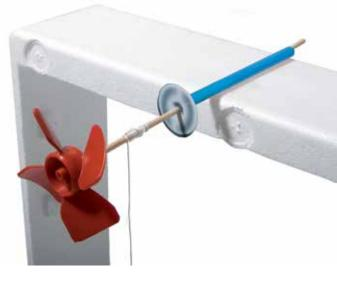
3. Tape some string between the propeller and disk. Then push the stick into the straw. 4. Tie the other end of the string to the black bottle. Blow on the propeller with your mouth or the hair dryer. The propeller will turn, winding up the string in the process and pulling the bottle upward. If the flow of air stops, the bottle drops down again and rotates the shaft and the propeller.
