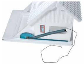
2. Open the two large windows and cut a section of yarn about 1 m in length. Tie one end to the angle gauge pointer, and the other end to a flashlight. Have an assistant shine the flashlight onto the house at a 60-degree angle, on the side of the house with the living room window. You will be able to tell by looking through the side window whether the flashlight beam is lighting the floor.
