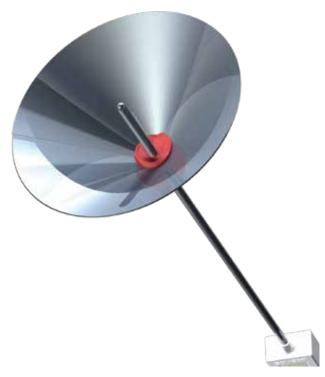
hold the thermometer body at the top. Watch the temperature. Within a few minutes, it will start to rise.
