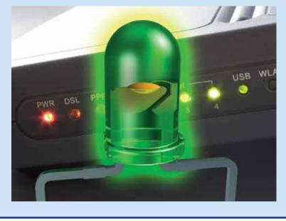
electricity flows. If it is connected the wrong way around, it will remain dark. LEDs have a few important advantages over conventional light bulbs: They use much less electricity for the same amount of brightness, and have a much greater life span.
