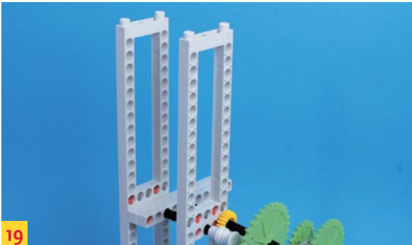
17 Now add a medium (17) and a long axle shaft (16) along with three small gear wheels (8).
