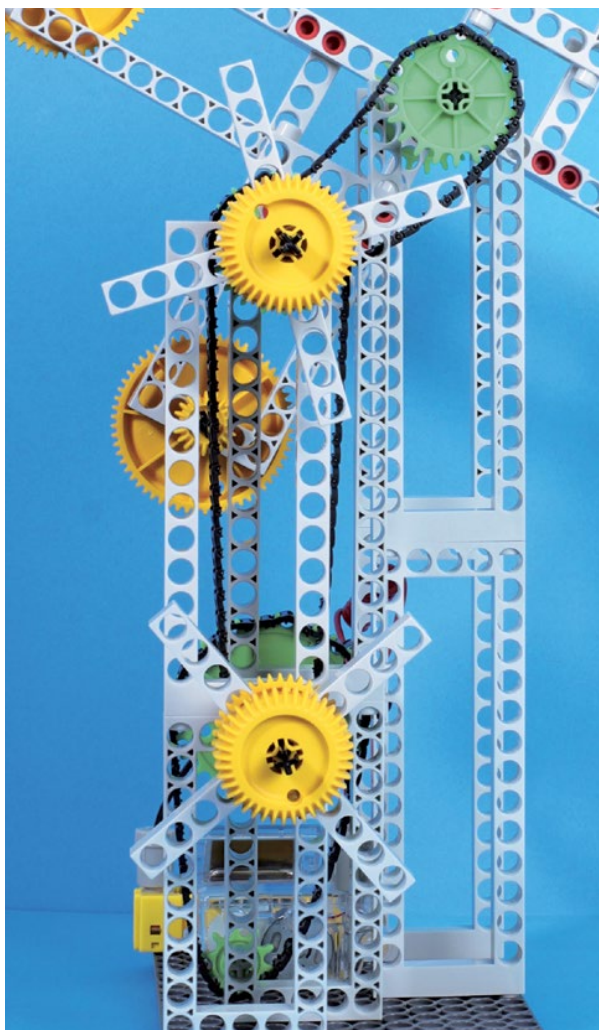
The solar engine drives not only the large windmill wheel in front, but also two small mill wheels on the rear side of the model.
