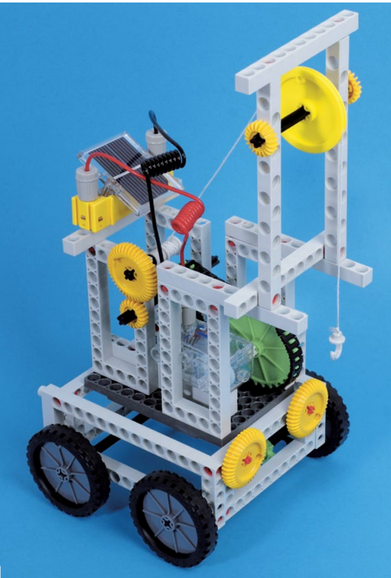
The crane car consists of two separated models: the crane assembly and the chassis it sits on.
