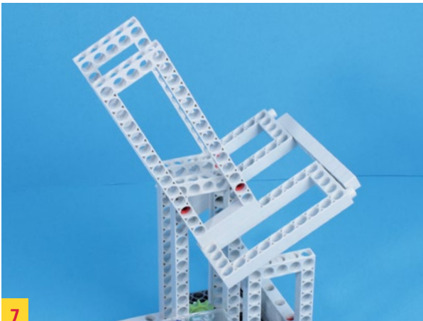
7 Now, attach two long frames (2) to the anchor pins. Attach a short frame (3) to the bottom of each of them, and connect the short frames at the rear with a short rod (4).
