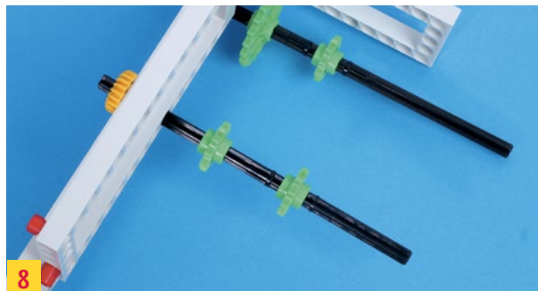
8 8. The drive shaft has to be lengthened too, although just with a medium axle shaft (17). The two shafts are held together with a small sprocket wheel (9).
