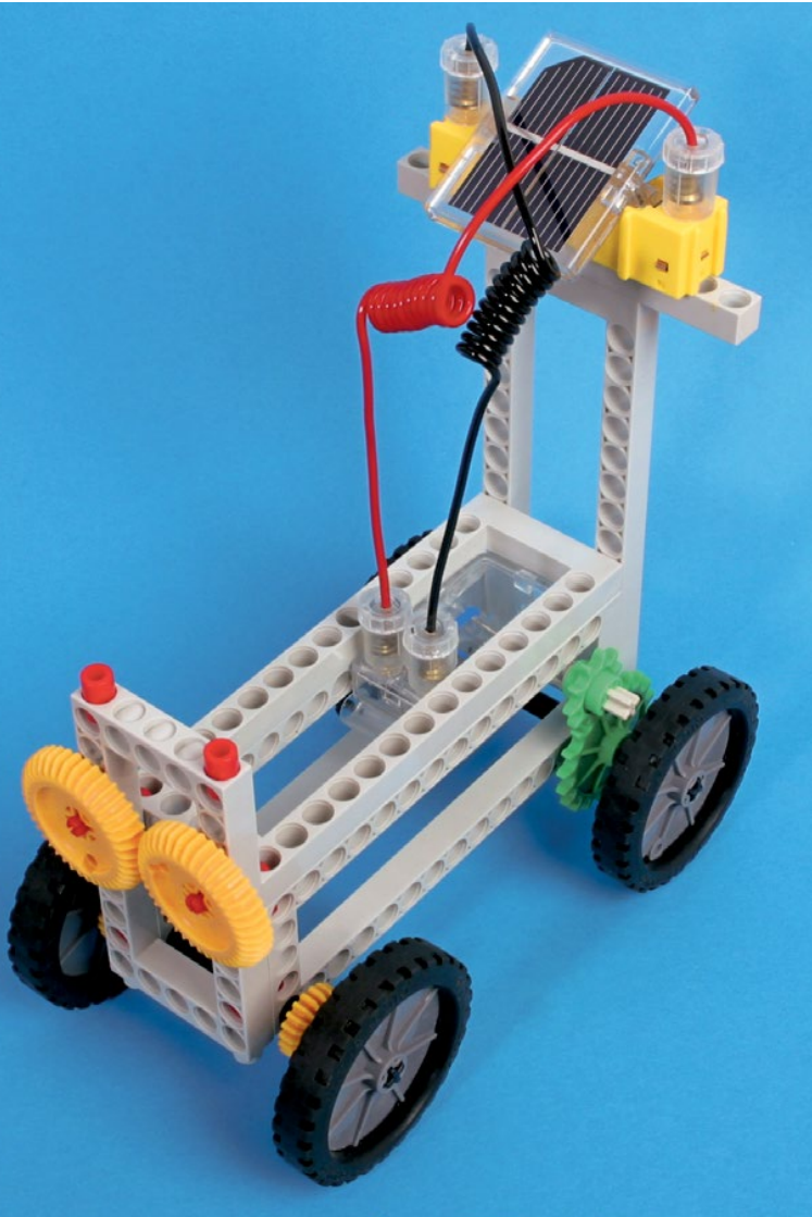
The solar tractor works with a gear drive. The small gear wheel on the engine turns the rear axle.
