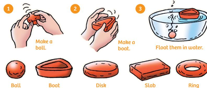
The clay boat and the clay ball weigh the same, but the boat displaces more water than the ball. Consequently, more water molecules press against the bottom of the boat, and it floats.
