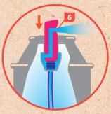
mixture inside the can. When the painter pushes down on the valve, the spring compresses and the channel opens. The high pressure gas Wants to push its way out of the can. As it does so, it carries the paint up the dip tube (5) and out the nozzle (6).
