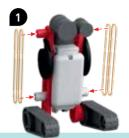
You can adjust the angle of Pogo's track-like feet. This means you can set the body to be more upright or more tilted forward. This affects Pogo's jump range. Test it out!
