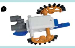
Scootz can also go in reverse. All you have to do is swap the position of the head and the ski so that the on/off switch is above the ski.
