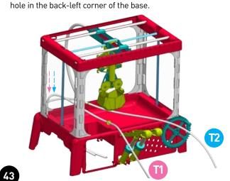
Connect the ends of tubes T1 and T2 that you fed though the hole to the hydraulic
