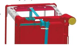
After completing step 43, turn the machine upright and test the movement of the claw from side to side by rotating the drive shaft (A1) in both directions. You may need to re-tighten the ribbon (step 43).
