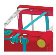
Then, slide the left spool to the right past the tab on P1. If you are having trouble pushing the spool past the tab, try pulling it away from the machine slightly as you move it.
