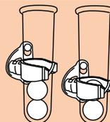
**Move pivot post down and tube up**
