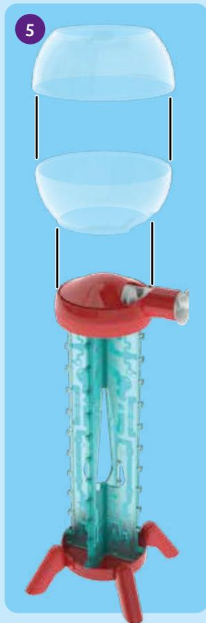
5 Put the bottom and top halves of the globe onto the globe base. Press them in securely. For an extra-secure closure of the two halves, you can use the **four clear rectangular stickers** provided. Apply them along the seam between the two halves.
