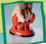
Because there are a lot more air particles per unit volume on the outside of the cup than there are on the inside, the air pressure is higher on the outside. This difference in air pressure is what keeps the suction cup stuck to the surface.
