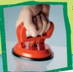
Because there are a lot more air particles per unit volume on the outside of the cup than there are on the inside, the air pressure is higher on the outside. This difference in air pressure is what keeps the suction cup stuck to the surface.
