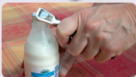
A bottle opener is a type two lever.
