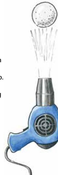
➤ **What's going on?** What's at work here is something called **Bernoulli's Principle**. It says that the pressure in flowing gases (or liquids) is lower than the pressure in ones that are still. So the ball is dancing in a region of lower air pressure. If it tries to break out to the side, the normal (higher) air pressure there pushes it back.
