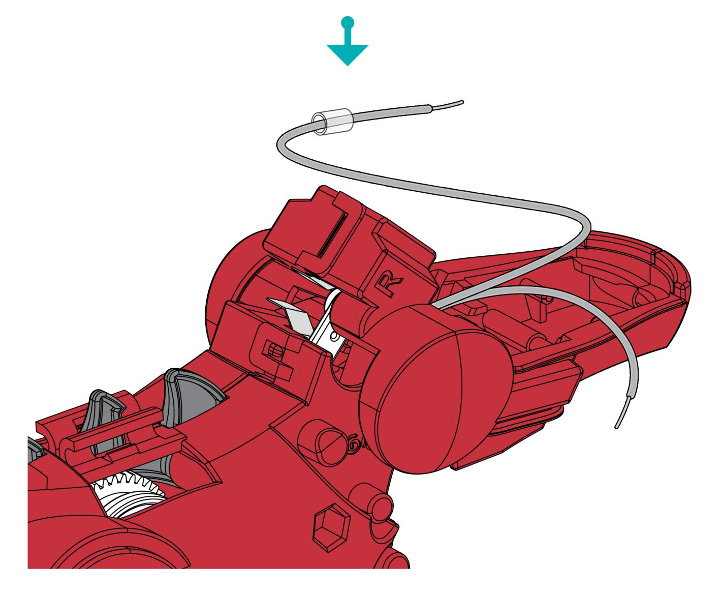
2.R Pass the metal end of the cable through the hole in the contact plate.
