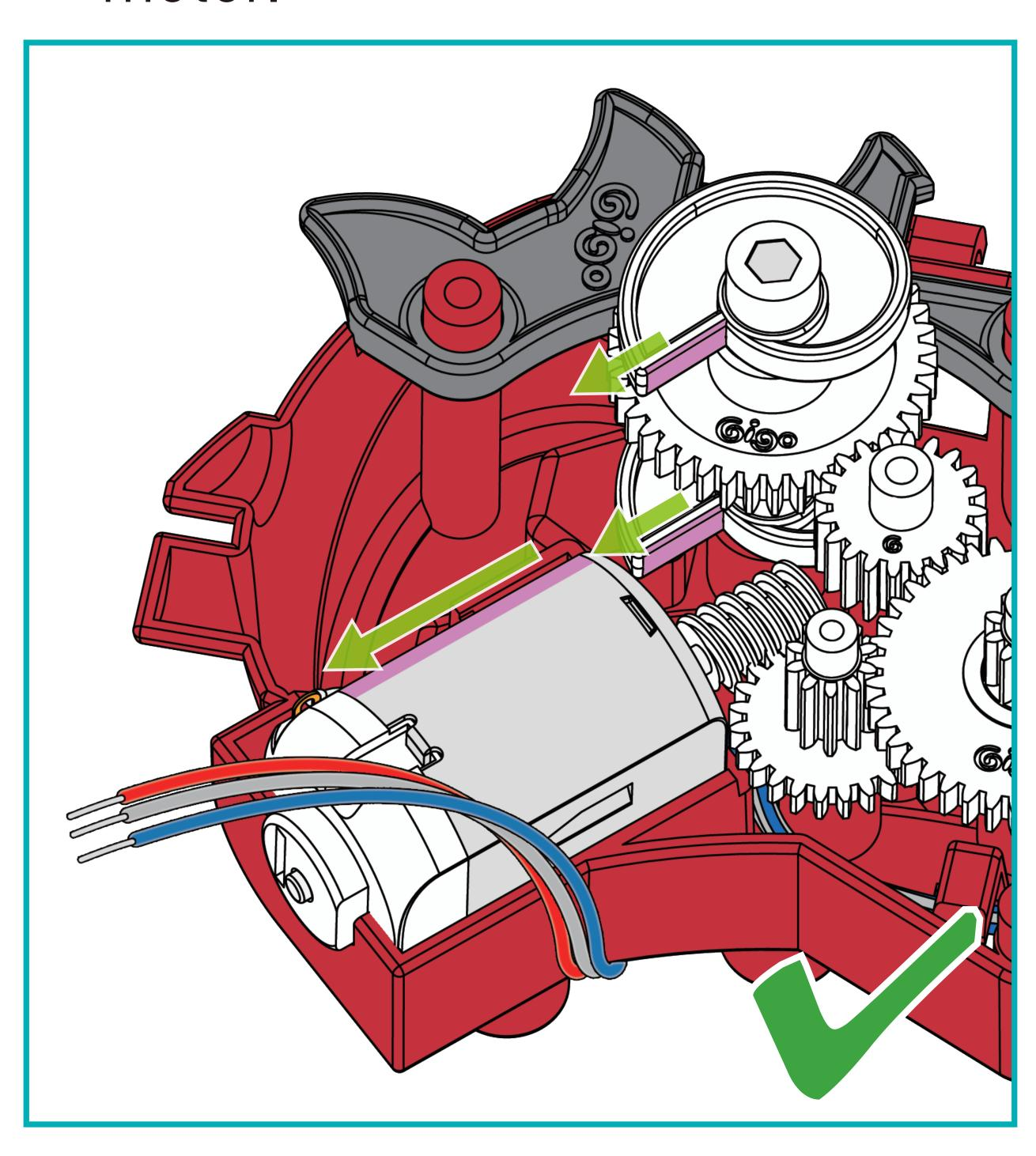
The tension rod is in the correct place and the blue cable is in the notch.
