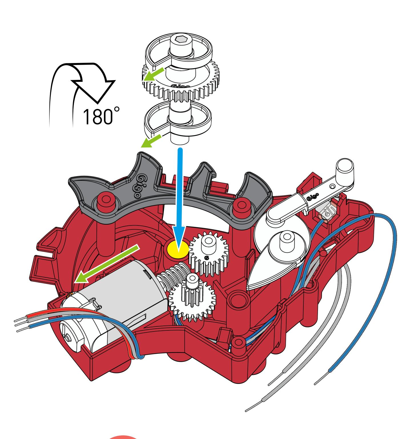
The straight edge of the cams must be parallel to the edge of the motor.
