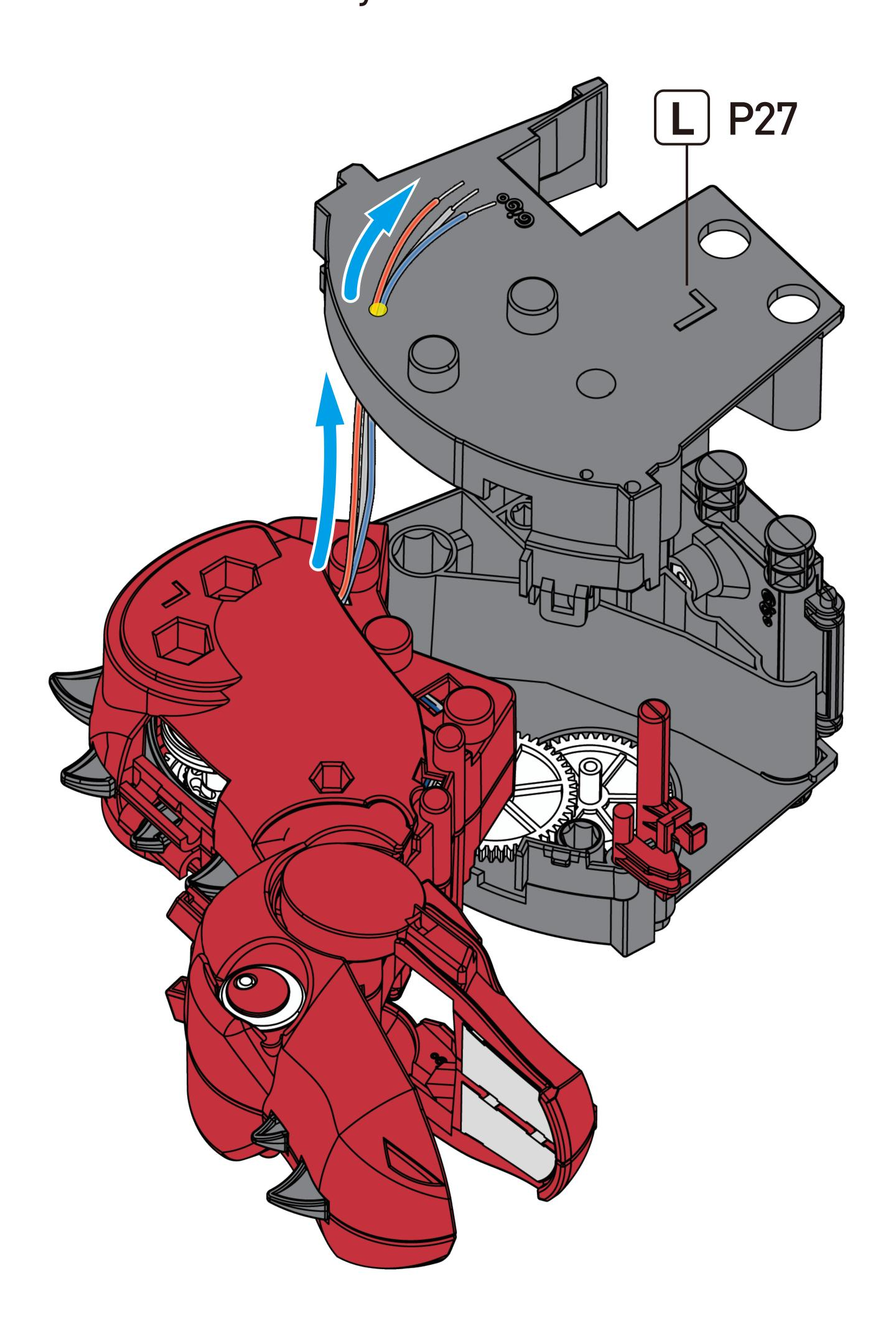
36 After assembling, pull the cables through as far as they go.
