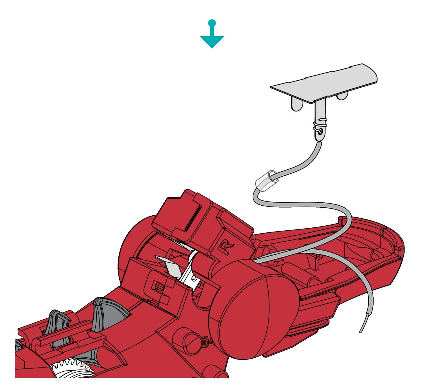
2.R Slide the contact protector on to the metal contact.
