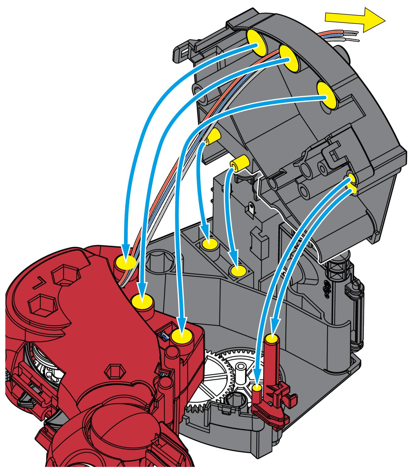
After assembly, no openings should be visible.
