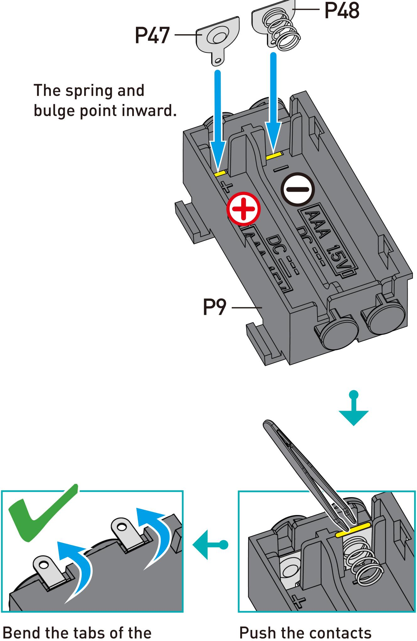
Bend the tabs of the contacts outward at a 90° angle.
