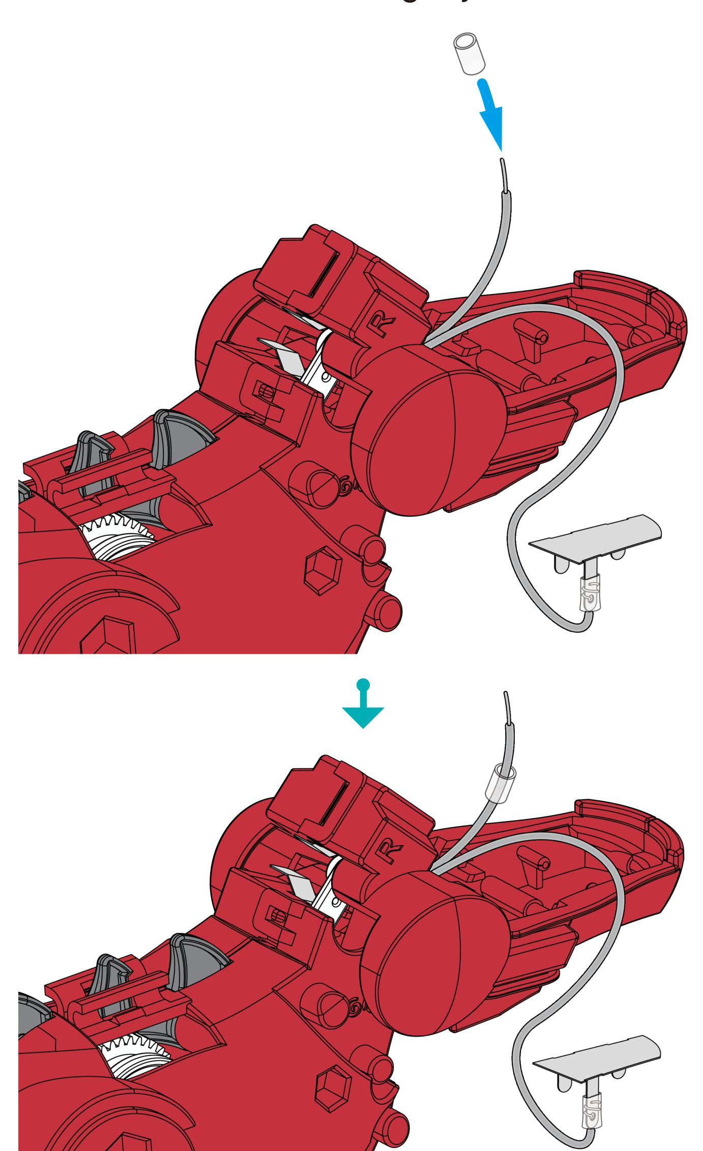
2.L Pass the metal end of the cable through the hole in the contact plate.
