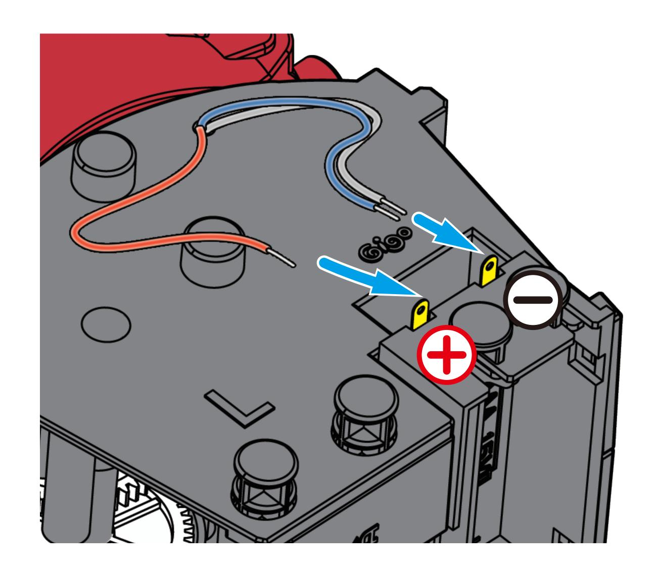
3. Slide the other contact protector on to the red cable. Connect the red cable to the positive contact.
