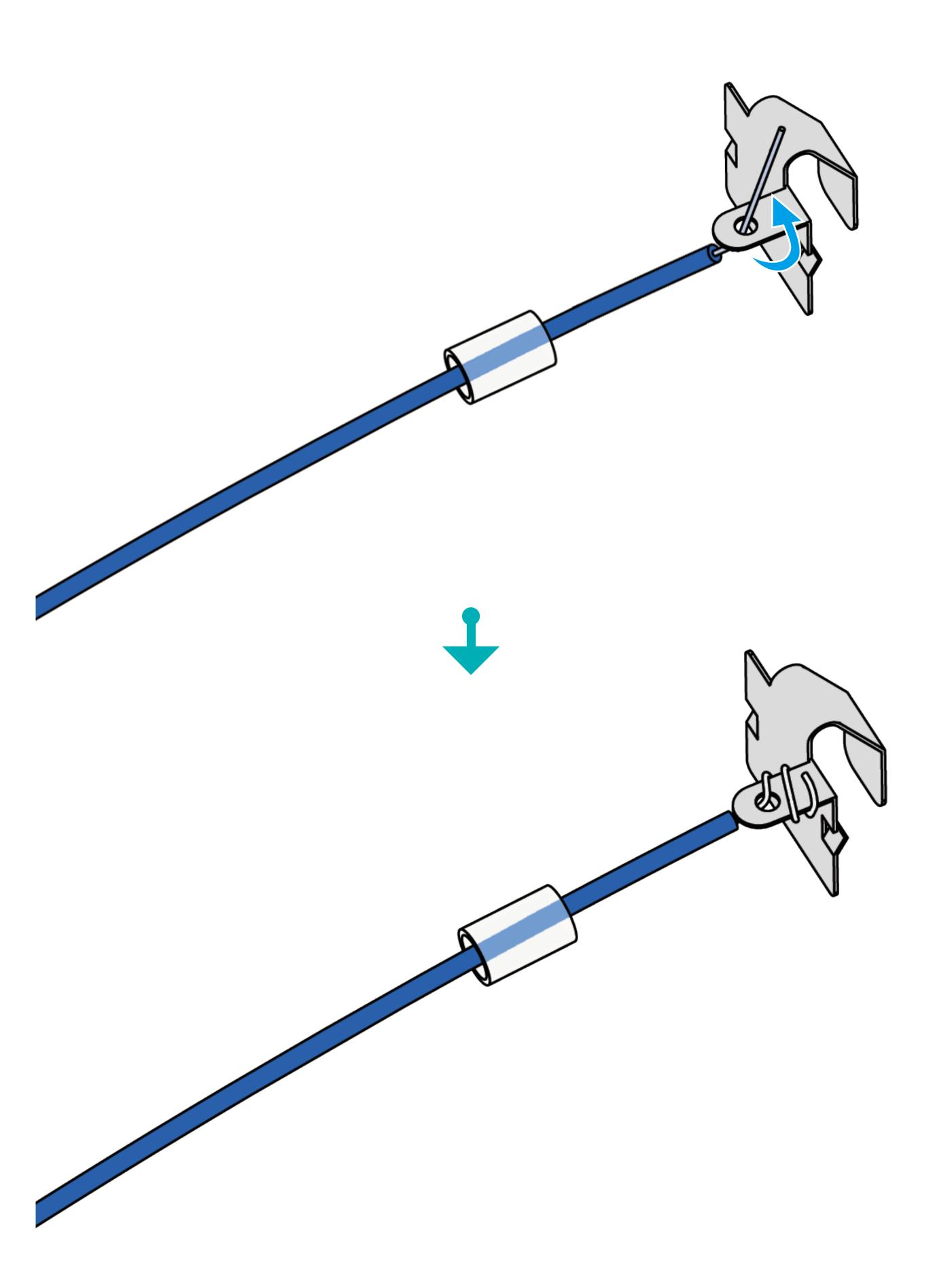
2. Slide the contact protector on to the metal contact.
