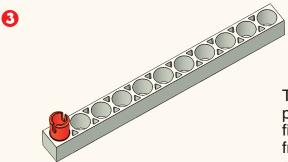
To remove a joint pin, pull it out with your fingers or push it out from the rear with the anchor pin lever.
