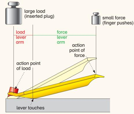
You cannot pull the plug out with your fingers, but the part separator tool can help you do it. It is a lever. The part of the lever that lifts the plug is shorter than the part you push on with your finger. With the long lever, you can pull out the plug with a small force. Some door handles are also shaped as levers. Can you think of other levers?
