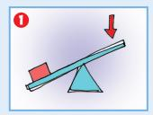
Lever: a bar that rests on a turning point that can be used to decrease the amount of force needed to move a load. Experiment 1. Examples: seesaw, crowbar, doorknob
