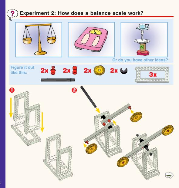
Here you have two levers. They are connected in the middle, at the point of rotation, like two arms. If both sides are loaded with the same weight, the scale is in balance. If you remove one gear wheel, the other side will be heavier and move downward.
