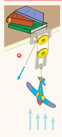
Two or more pulleys can be put together into a device called a block and tackle. The simplest version has a fixed pulley, like the one from the previous experiment, and a moving pulley attached to the load. When lifting the load, you will notice that you are changing the direction of the force. You are pulling down instead of up. And when pulling, you can feel that you need far less force than the weight of the load.
