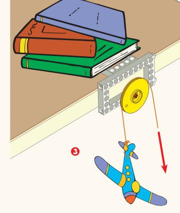
Pulleys can be found everywhere. They are used in places where the direction of a force must change, for example on elevators, construction sites, or onboard sailboats. In the experiment, you were able to move your toy upwards by pulling downwards on the string. You will need exactly the same force as without a pulley, but the direction of the force is changed. This is how a construction worker standing on the ground can easily get materials to his coworker above.
