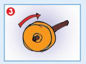
Wheel and Axle: a lever that turns in circles around a point, which can decrease the amount of force needed to move a load. Experiments 5 and 7. Examples: wheels on a car, gears on a bike
