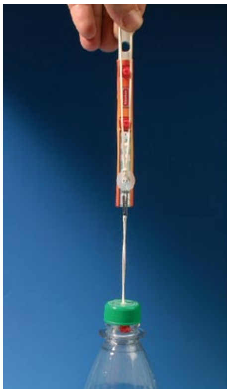
Your force meter can measure the weight that pulls on the bottle. Thus, it functions as a scale.
