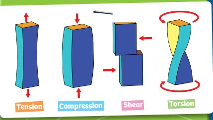
Structural engineers often use four terms to describe how a load can affect a structure: tension, compression, shear, and torsion.
