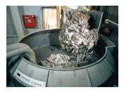
giant stirring bowl. This thin pulp is taken from the supply vat onto a movable screen. The movement helps the fibers to intertwine as tightly as possible. In the process, most of the water runs off. Then, the web of soaked paper comes to the press. The paper web is guided through rollers in an absorbent felt
