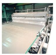
cloth and the rest of the water is thereby removed. This pressing process makes the paper structure denser and firmer. Then, the paper web runs through heated drying cylinders. Finally, it is smoothed and rolled up.
