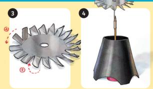
3. Press the cut tealight cup wall flat and bend one edge of each blade slightly up.
