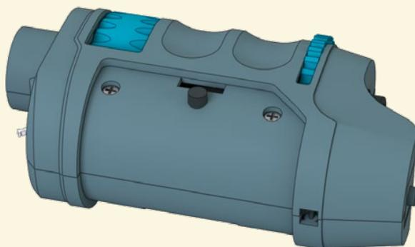
The basic assembly is now complete. Check the functioning of the zoom and focus adjustment wheels.
