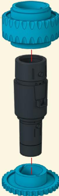
The zoom adjustment wheel is mounted on the top. This will be used to move the relay lens and adjust the zoom setting between 20-fold and 40-fold magnification.
