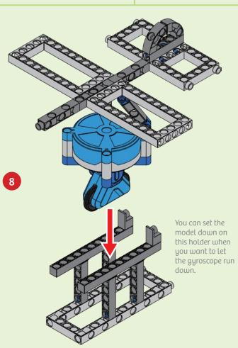
Remember that the gyroscope has to be switched on if you want the model to balance.
