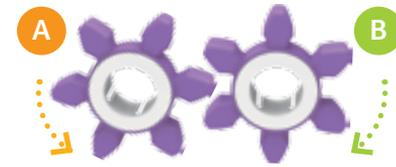
When **gear A** turns around once, **gear B** turns around once. They both have six teeth. This gear spins freely on a dowel.
