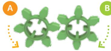
When **gear A** turns around once, **gear B** turns around once. They both have six teeth.
