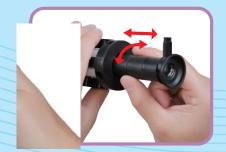
Slowly rotate the eyepiece tube to push it inward or slide it outward.
