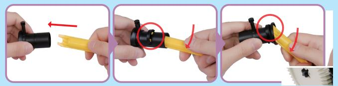
Insert the tool into the eyepiece tube.
