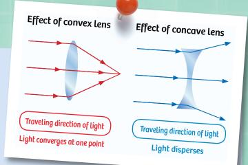
convex lens causes straight rays of light to converge,
