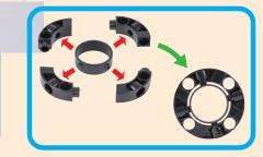
5. Make sure the four pegs on the tube ring are completely inserted into the four holes in the bent rods.
