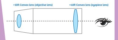
Add an extension tube to try a longer microscope! What is the size and brightness of the image viewed by the longer microscope?
