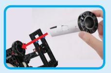
5. Insert the tube through the frame and partially into optical tube C.
