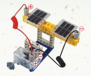
Fig. b. You can also connect the two solar panels in series as shown here.
