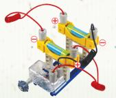
Fig. h. You can connect two fully charged AA batteries in series like this.
